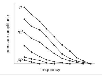
FIGURE 8. The internal spectrum of a brass instrument, for a range of air-pressure levels, after Benade (1990).
