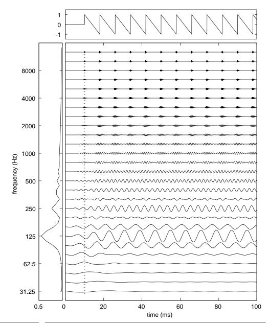
**FIGURE 20.** Response of the cochlear filter bank *with* group-delay compensation. The output of every second filter channel is shown. The left panel shows the RMS amplitude of the filters as a function of center frequency. The top panel shows the sawtooth waveform to illustrate the alignment of the amplitude-modulation peaks. Note the improved vertical alignment in comparison with Figure 19.
