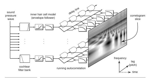
FIGURE 23. Block diagram of the calculation of the correlogram, after Ellis (1996).
