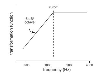
FIGURE 9. Schematic of the bell transformation function for a trumpet, after Benade (1990).
