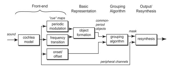
FIGURE 2. Overview of processing flow in CASA architectures, after Ellis (1996).
