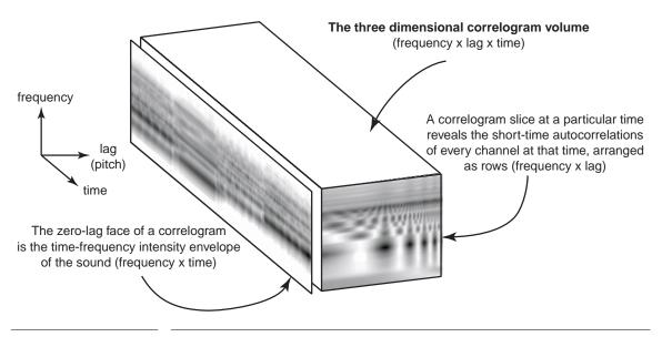
FIGURE 22. Illustration of the correlogram volume, after Ellis (1996).
