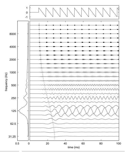
**FIGURE 19.** Response of the cochlear filter bank *without* group-delay compensation. The output of every second filter channel is shown. The left panel shows the RMS amplitude of the filters as a function of center frequency. The top panel shows the sawtooth waveform to illustrate the alignment of the amplitude-modulation peaks.
