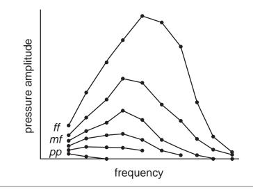
FIGURE 10. The external spectrum of a brass instrument, for a range of air-pressure levels, after Benade (1990).
