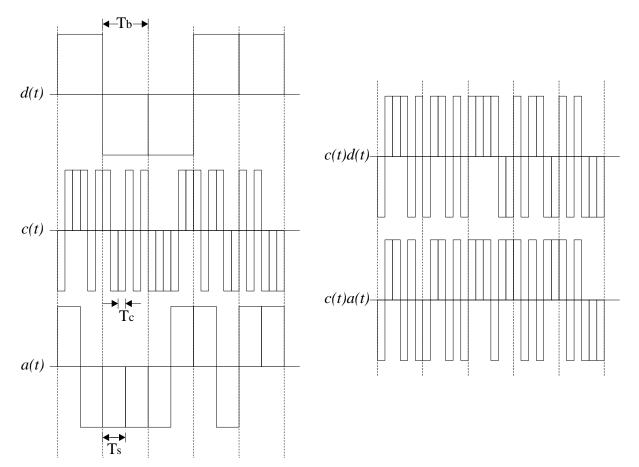
Figure 11. Coded and uncoded signals before spreading
