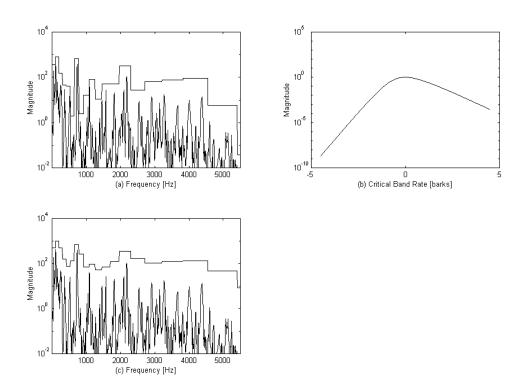
Figure 26. (a) Energy per critical band Spz(z), (b) spreading function B(z), and (c) Spread energy per critical band Sm(z)
