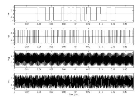
Figure 23 Time domain signals: data bit stream, d(t); PN sequence, c(t); BPSK modulator, sin(t); and watermark audio signal, x(t)
