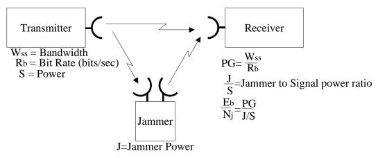
Figure 5. Basic spread spectrum communications system
