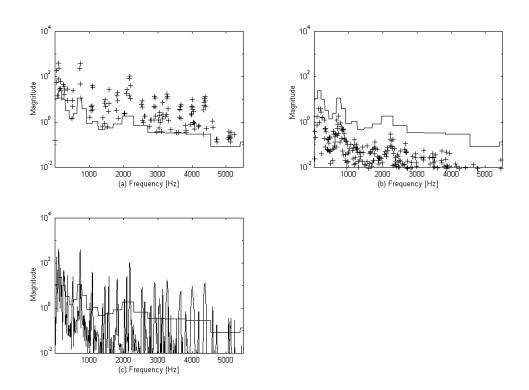
Figure 29. Final masking threshold Tfinal(z), and the power spectrum of (a)  $Swnew(j\mathbf{W})$ , (b)  $Xfinal(j\mathbf{W})$ , and (c)  $OUT(j\mathbf{W})$ .
