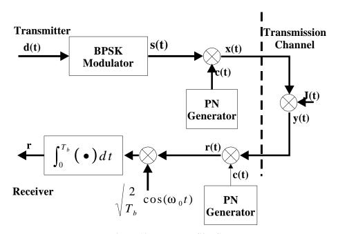
Figure 10. Uncoded DS/BPSK
