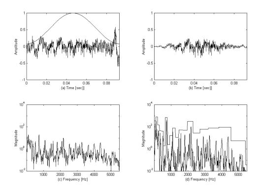
Figure 25. (a) Audio signal s(t) and window signal w(t), (b) windowed signal sw(t), (c) magnitude of frequency representation  $Sw(j\mathbf{W})$ , and (d) power spectrum  $Sp(j\mathbf{W})$  and energy per critical band Spz(z)
