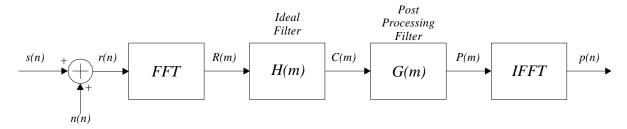
Figure 15. FFT filter assuming additive signal and noise
