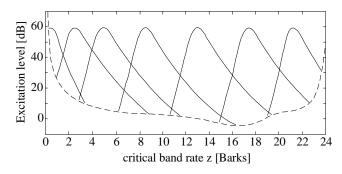
Figure 3. Excitation level versus critical band rate for narrow band noises with various center frequencies [1]
