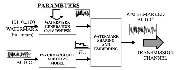
Figure 16 Proposed system (watermark generation and embedding)
