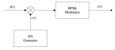
Figure 8. DS/BPSK modulation
