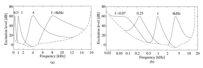
Figure 2. Masking curves in (a) linear and (b) logarithmic frequency scale [1]
