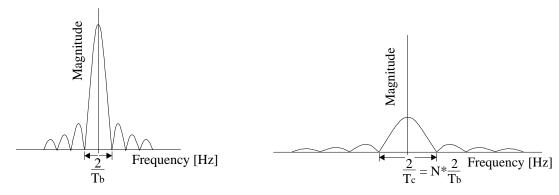
Figure 6. Spectrum of signal BPSK
